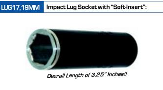
This is the Real Deal! You won't find a stronger, more durable impact socket equipped with an aluminum "Soft-Insert". It is designed so as not to damage, scuff or mar expensive, highly polished steel or aluminum Lug Bolts which are generally found on Porsche, BMW, Mercedes, etc. Its length allows for easy access to lug bolts on extra wide rims.
