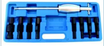
This Porfessional Master set is the most extensive and precise **(8)** piece Blind Hole Bushing and Bearing Puller set ever assembled. All pieces of this master kit have their own compartment within in a blow mold storage case.
