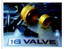
Due to the close proximity of transversely mounted engines to the shock tower, this essential tool is crucial for the proper installation of **Cam Shaft**Oil Seals. Comes equipped with an exclusive expansion guide ensuring damage free installation.
